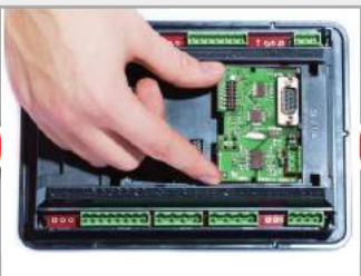
INSERT THE PLUG&PLAY EXPANSION MODULE INTO ONE OF THE TWO SLOTS
